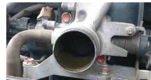
BEFORE (Throttle body condition after 60,000 km)
