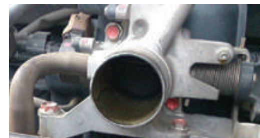
BEFORE (Throttle body condition after 60,000 km)
